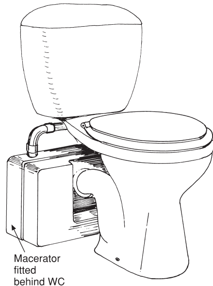
Fig. 7.1 Pictorial illustration of WC suite fitted with macerator unit.
